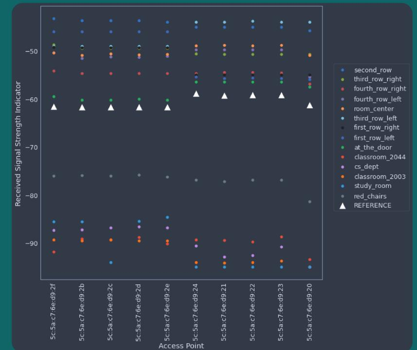
**Figure 2.** Top 10 Access Points by MAC address versus average RSSI. The points labeled as “Reference” represent the RSSI from a fixed location in the classroom used as a basis of comparison for the other recorded locations — in and outside of the classroom, but in the same building.
